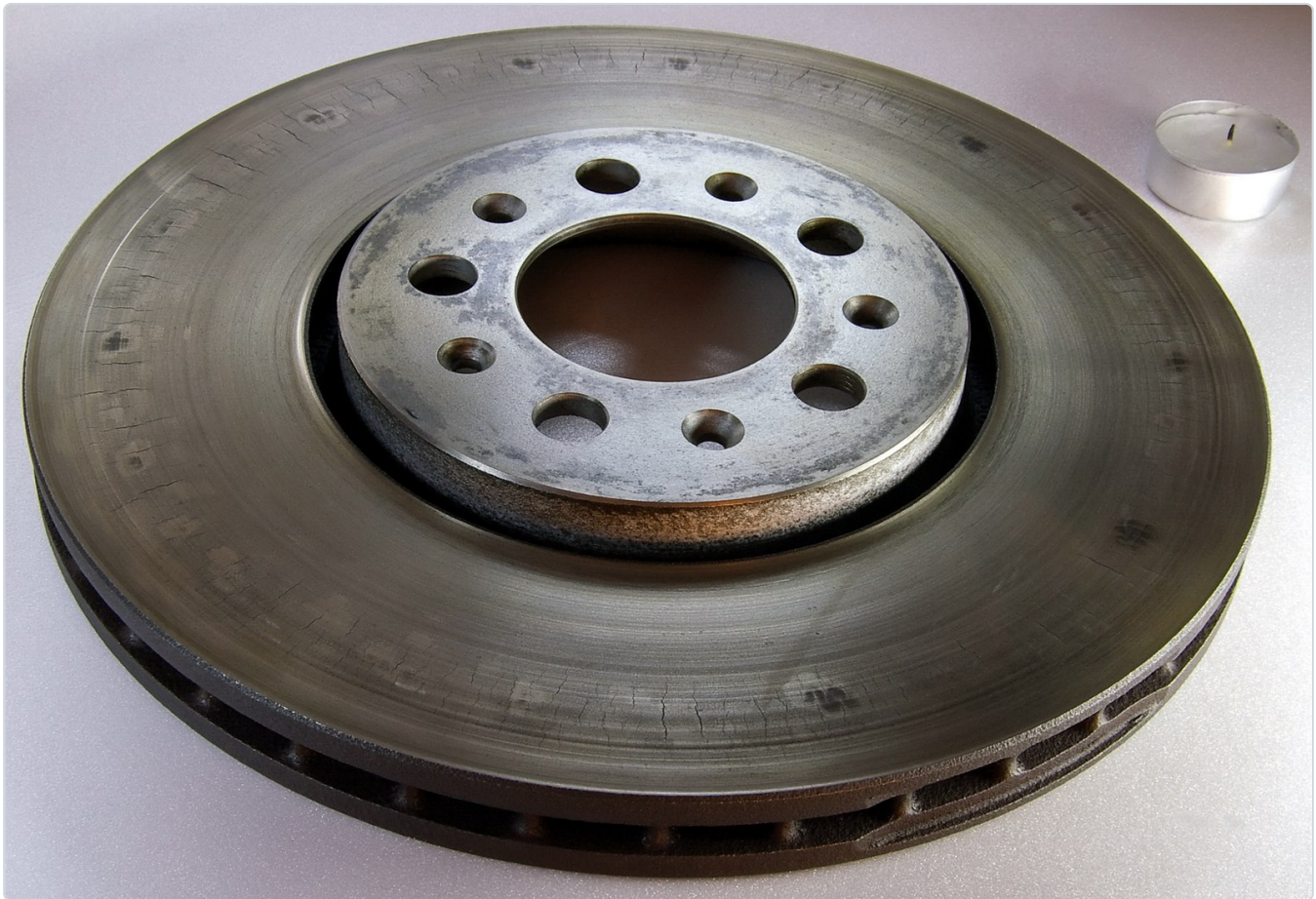
A worn-out brake rotor. The surface is grooved and cracked from heat and metal rubbing on it. A rotor like this needs replacing, not resurfacing.
