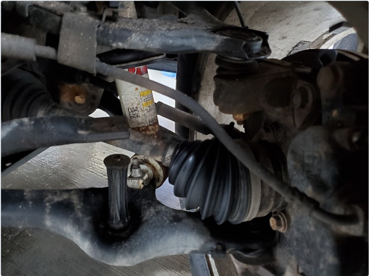
A broken sway bar end link under the car. This small rod with a joint at each end is the cheapest and most common cause of a clunk over bumps.
