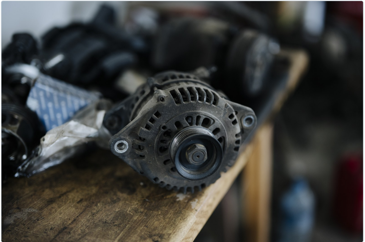
A car alternator sitting on a workbench, seen from the pulley end. The belt rides on the grooved pulley in the middle, and the slots in the housing let air through to cool the windings inside.
