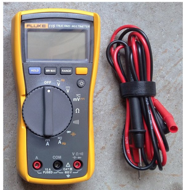
Two-lead digital multimeter with test leads, rated CAT III 600 V
