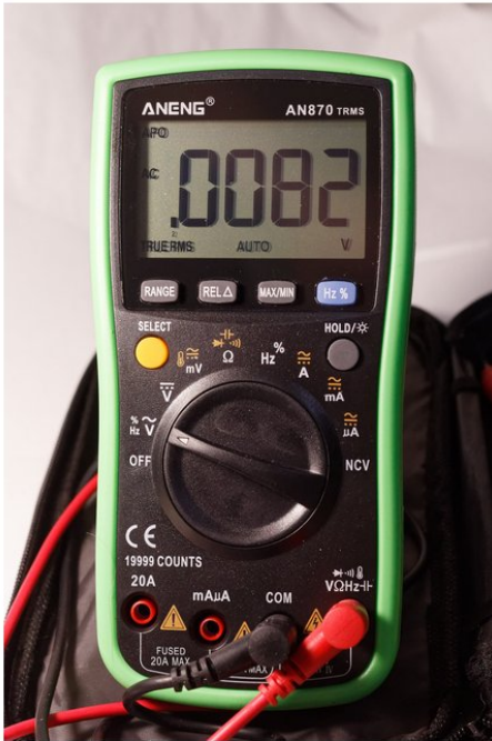
Knob on AC volts (V~). Black lead in COM, red lead in V.
