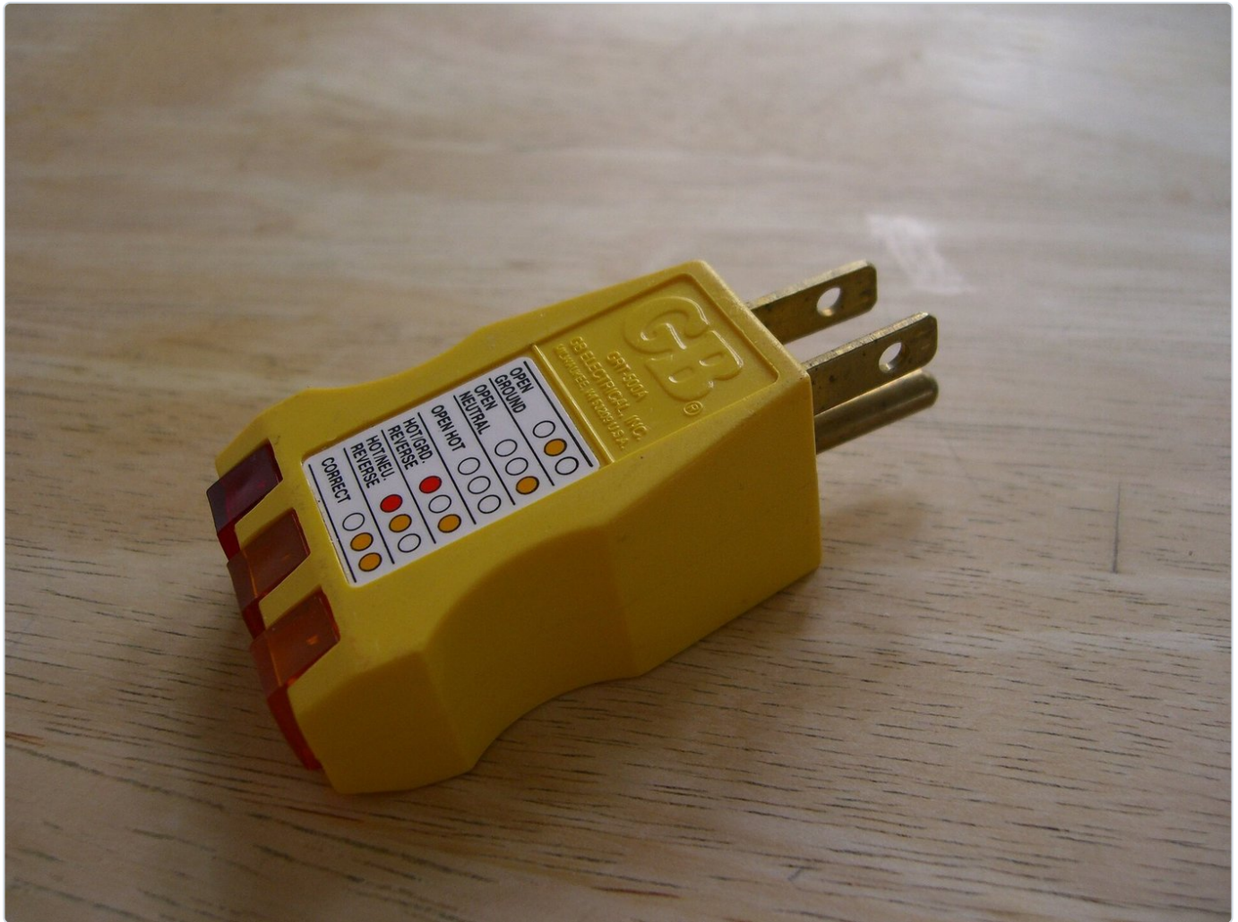
A plug-in receptacle tester. The chart on top shows which pattern of the three lights means correct wiring and which means open ground, open neutral, open hot, or reversed hot and neutral.
