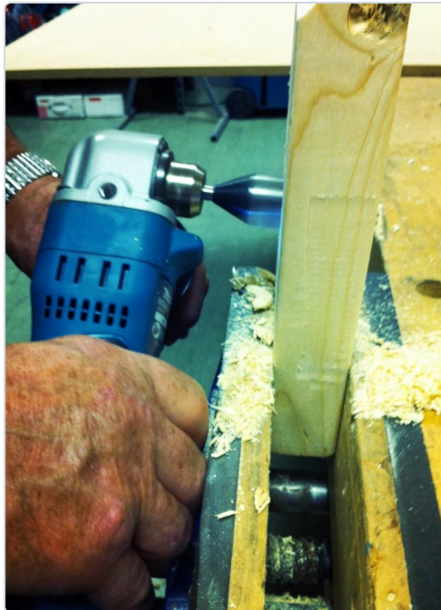
A right-angle drill boring through a stud with a self-feed bit. The short head lets the drill fit between studs and joists where a normal drill will not go.
