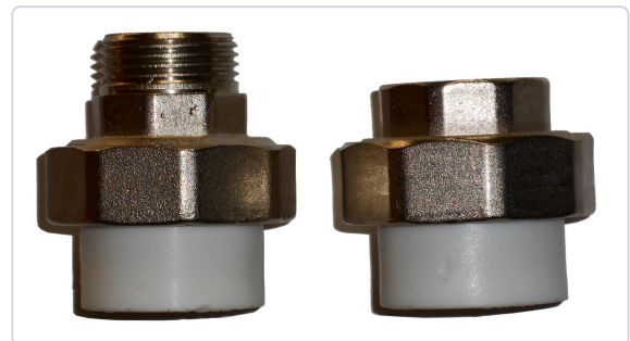
Two unions (male-thread and female-thread). The big nut in the middle lets you take the joint apart later without turning either pipe.
