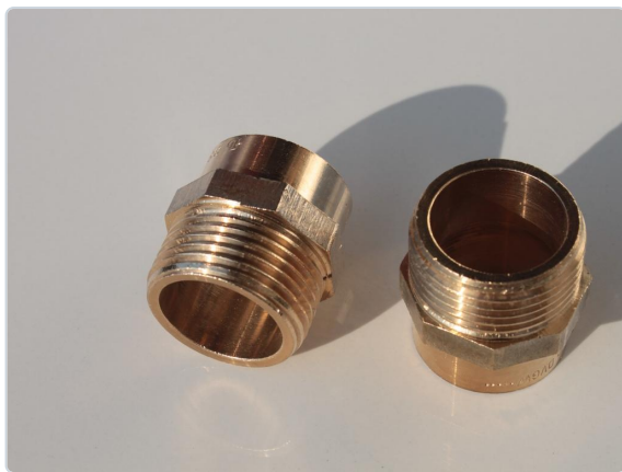
Two male adapters: the smooth end is soldered onto copper tube and the threaded end screws into a female fitting.
