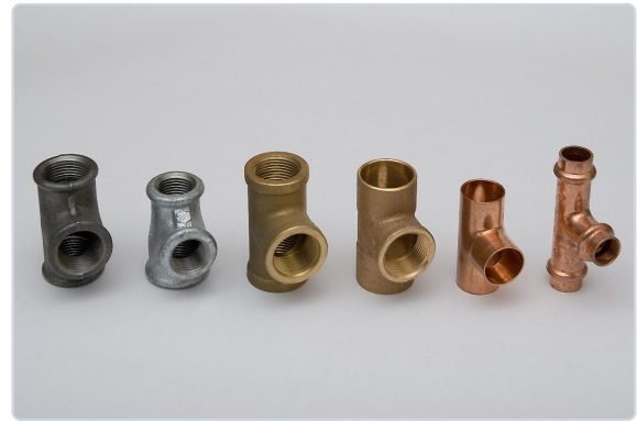
The same tee in six materials, left to right: black malleable iron, galvanized iron, brass threaded, bronze threaded, copper sweat, copper press.
