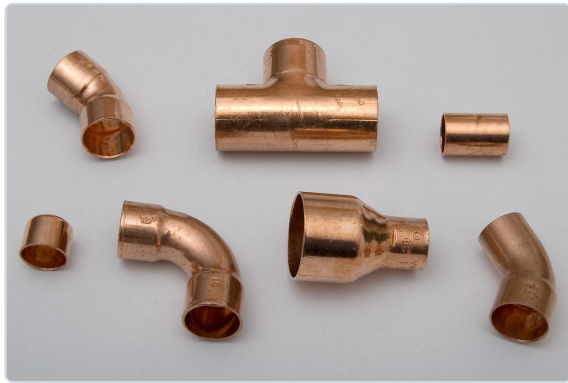
Copper sweat fittings. Top row: 45-degree elbow, tee, coupling. Bottom row: cap, 90-degree elbow, reducer, street 45 (one end fits inside a fitting).
